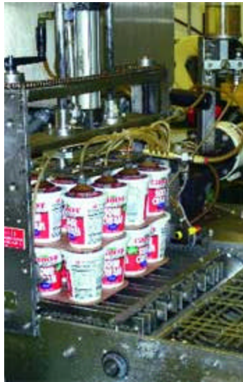
Cabot's retail products are unitized using a construction of corrugated pads and shrink wrap that eliminates the need for trays or cases.
