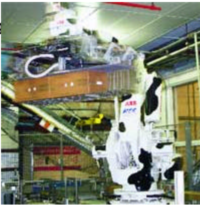
Cabot's retail products are unitized using a construction of corrugated pads and shrink wrap that eliminates the need for trays or cases.
