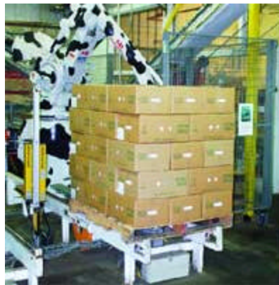
Completed pallet loads are conveyed out of the palletizing cell, where they wait for transport by forklift to Cabot's distribution cooler.
