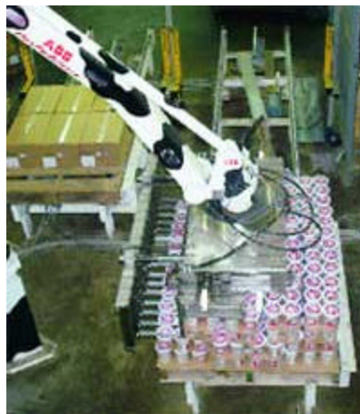
A custom-designed mechanical gripper arm enables the robot to gently handle shrink-wrapped multipacks at high throughput speeds.
